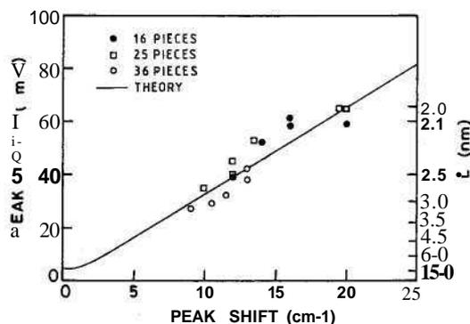
Fig. 3. Peak width vs. peak shift of the first-order Raman peak for nanocrystals with different Si/SiO<sub>2</sub> compositional fraction and annealed at different temperatures and durations. The solid line is theoretical curve calculated using the phonon confinement model with the Gaussian weighting function. The right ordinate shows the dimension of the nanocrystals.
