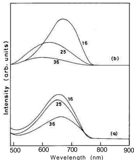
Fig. 6. A comparison of room temperature PL spectra from samples having different Si/SiO<sub>2</sub> compositional fraction; (a) as-deposited sample (b) annealed at 980 °C, 2 h.
