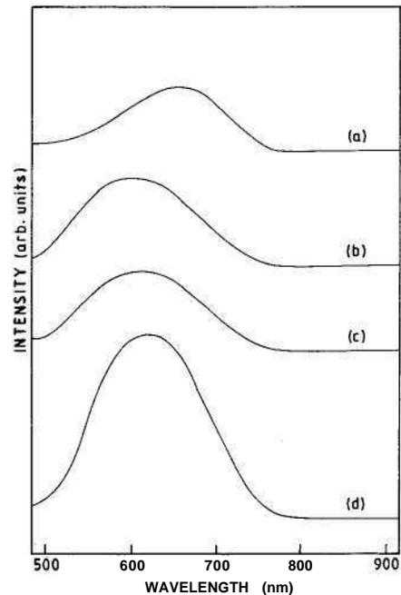
Fig. 5. Room temperature PL results from the nanocrystalline silicon samples produced by RF sputtering with 36 Si pieces on the sputtering target; (a) As deposited and annealed in argon at temperatures 1000 °C for a duration of (b) 30 min (c) 1 h (d) 2 h.
