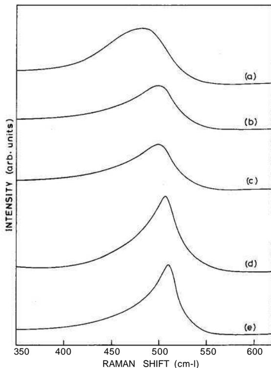
Fig. 1. First-order Raman spectra from the nanocrystalline silicon samples produced by RF sputtering with 25 Si pieces on the sputtering target and annealed in argon at temperatures (a) 900 °C, (b) 930 °C, (c) 950 °C, (d) 980 °C, (e) 1000 °C for a duration of 2 h.
