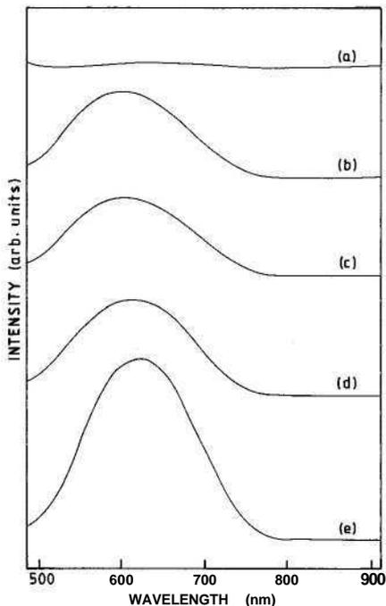
Fig. 4. Room temperature PL results from the nanocrystalline silicon samples produced by RF sputtering with 36 Si pieces on the sputtering target and annealed in argon at temperatures (a) 900 °C, (b) 930 °C, (c) 950 °C, (d) 980 °C, (e) 1000 °C for a duration of 2 h.
