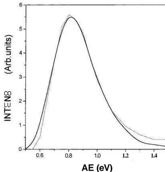
Fig. 7. The dashed curve shows the room temperature PL spectrum from the sample (16 piece) annealed at 1000 °C for 2 h. The solid line shows the theoretical fit to the experimental curve.
