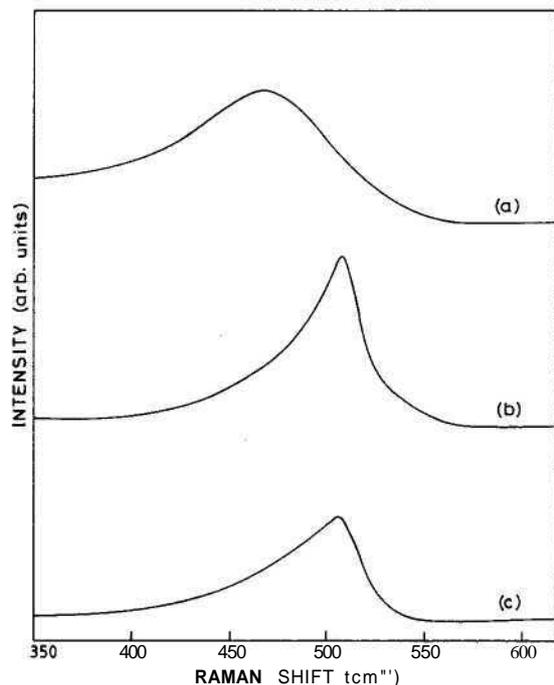
Fig. 2. First-order Raman spectra from the nanocrystalline silicon samples produced by RF sputtering with 25 Si pieces on the sputtering target (a) as deposited and annealed in argon at 1000 °C for duration of (b) 1 h (c) 30 min.
