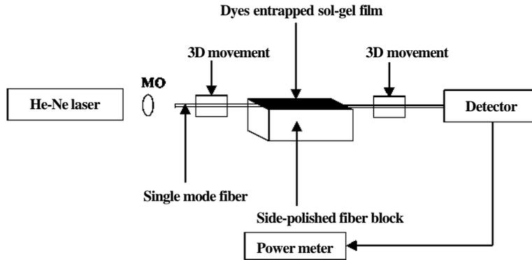
Fig. 3. Experimental set up of the fiber optic pH sensor based on side-polished single mode optical fiber half block.
