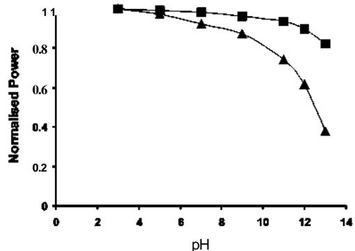
Fig. 4. Calibration curve of the side polished single mode optical fiber pH sensor for half blocks with radii of curvature of the grooves 22 cm (N) and 25 cm (j).
