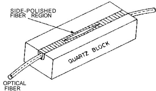
Fig. 2. The schematic diagram for the side-polished single mode optical fiber half block.
