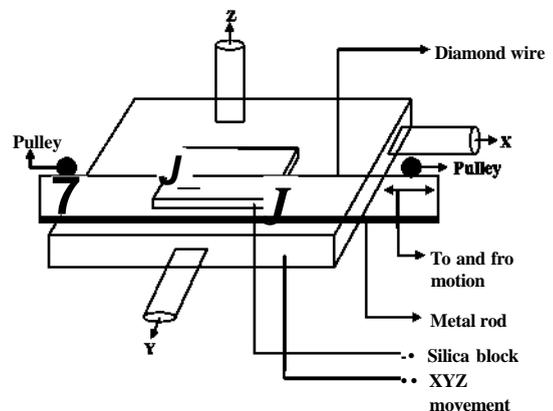
Fig. 1. The schematic diagram for the machine used to make the groove of desired radius of curvature on a silica/quartz block.
