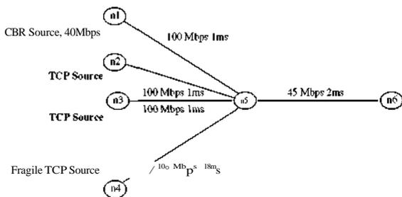
Fig. 15. Simulation scenario with a fragile flow.
