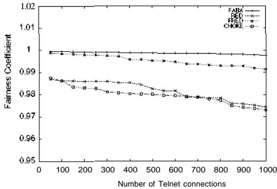
Fig. 14. Fairness coefficient versus number of Telnet connections for different AQM schemes.
