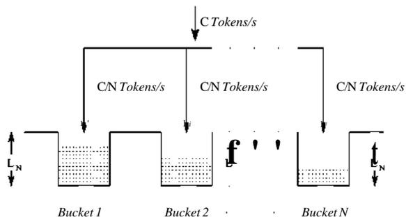
Fig. 2. FABAs architecture for rate control using token buckets.
