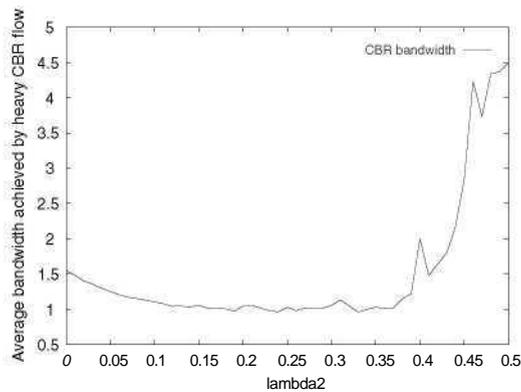
Fig. 4.  $k_2$  versus average bandwidth achieved by heavy CBR flow.
