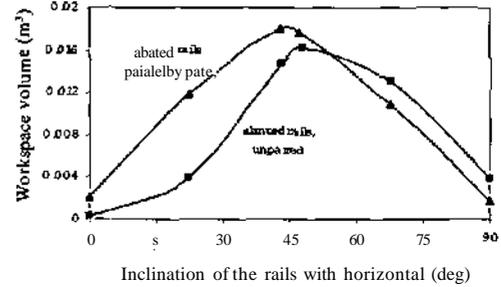
Fig. 6(a) Variation of workspace with the rail inclination
