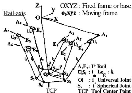
Fig. 1 The general hexaslide machine tool
