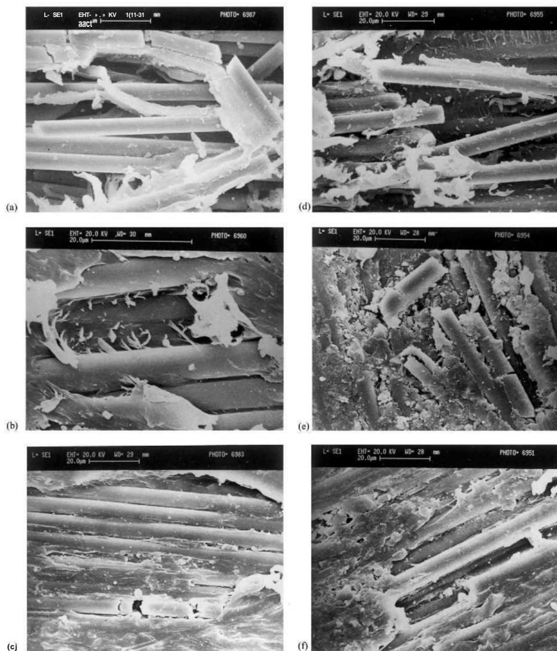
Fig. 6. Scanning electron micrograph of surfaces eroded at impingement angle of  $15^\circ$  with steel balls of diameter 300-500  $\mu\text{m}$ . Impact velocity is 45 m/s for (a-c) and 85 m/s for (d-f), respectively ((a) and (d)  $90/0-0^\circ$  fibre orientation; (b) and (e)  $90/45-45^\circ$  fibre orientation; (c) and (f)  $90/90-90^\circ$  fibre orientation).
