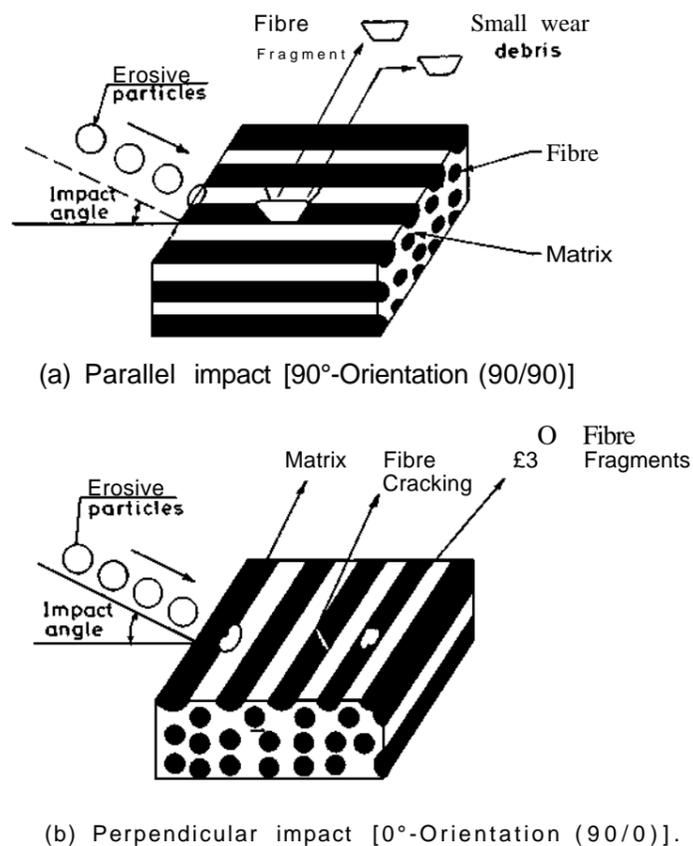
Fig. 5. Schematic diagrams of erosive process in unidirectional fibre reinforced composites under parallel and perpendicular impact conditions.
