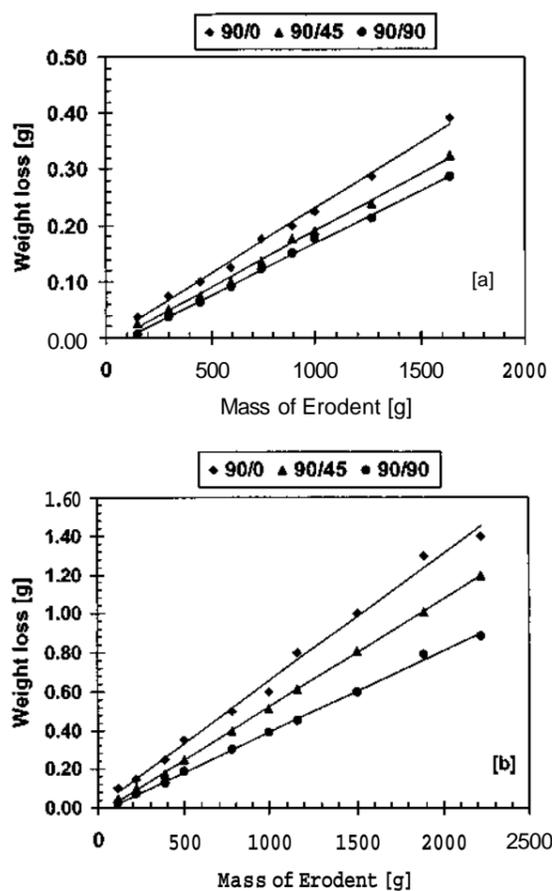
Fig. 3. Variation of erosive wear with mass of erodent for different impact velocity ( $V$ ): (a) 45 m/s; (b) 85 m/s; (impingement angle = 60°; exposure time = 180 s).
