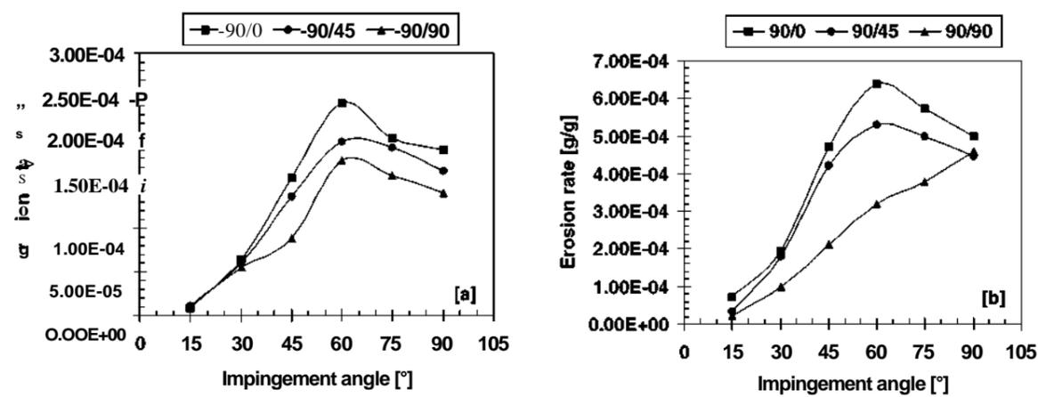
Fig. 4. Variation of normalised erosion rate with impingement angle for three fibre orientations: (a) impact velocity ( $V$ ) 45m/s; (b) 85m/s (exposure time = 180 s).
