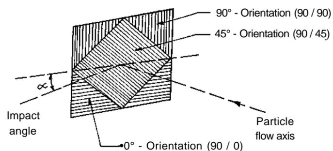
Fig. 2. Definition of impingement angle and fibre orientation.
