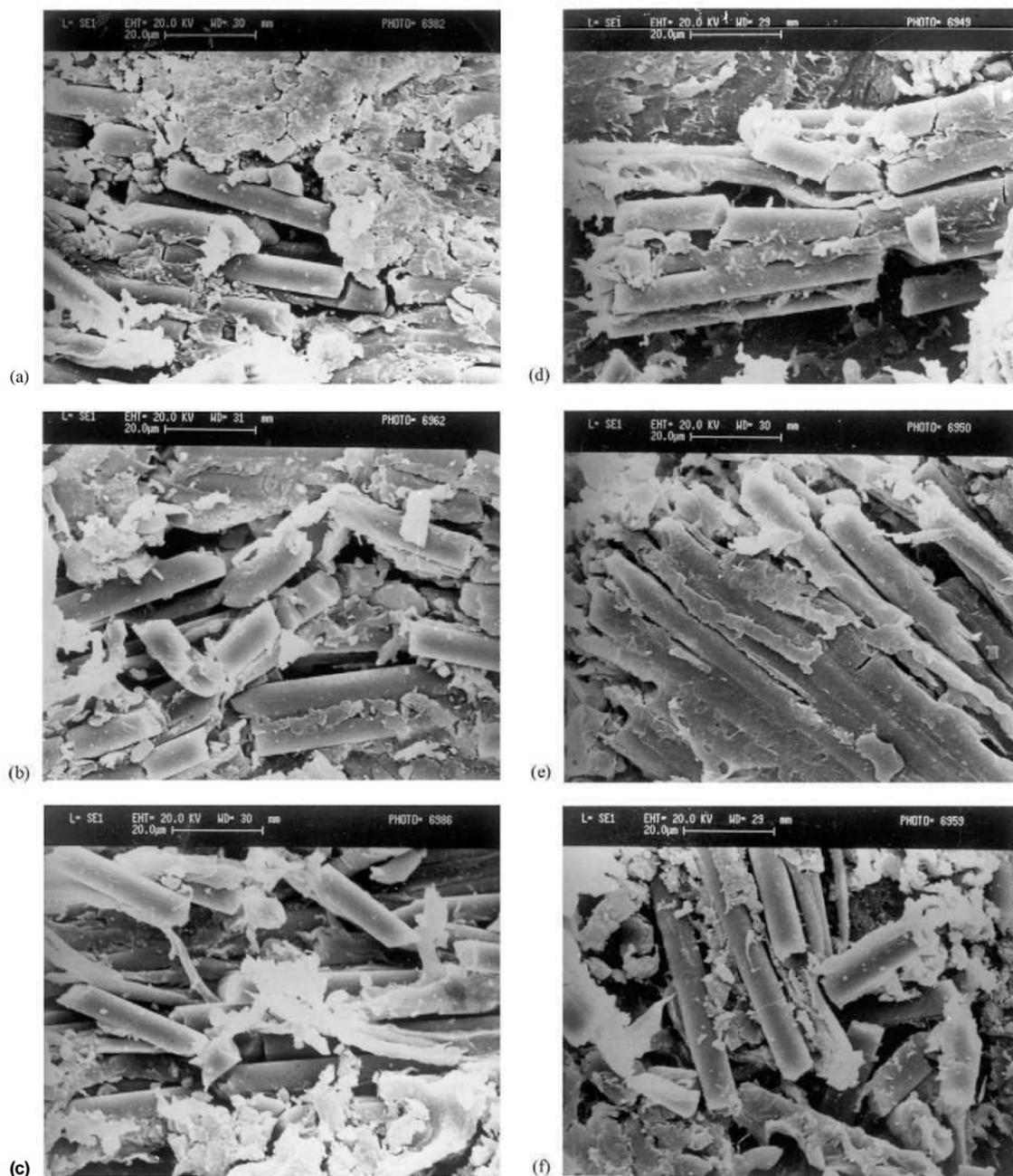
Fig. 7. Scanning electron micrograph of surfaces eroded at impingement angle of  $60^\circ$  with steel balls of diameter 300-500  $\mu\text{m}$ . Impact velocity is 45 m/s for (a-c) and 85 m/s for (d-f), respectively ((a) and (d)  $90/0-0^\circ$  fibre orientation; (b) and (e)  $90/45-45^\circ$  fibre orientation; (c) and (f)  $90/90-90^\circ$  fibre orientation).
