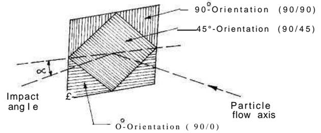
Fig. 2. Definition of impingement angle and fibre orientations.
