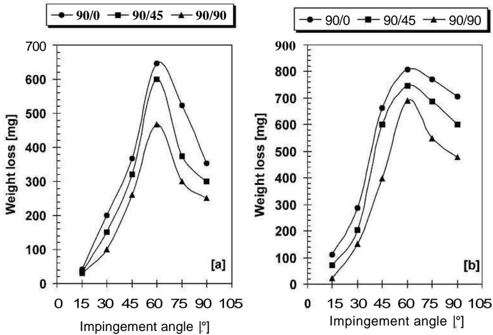
Fig. 4. Influence of impingement angle, fibre orientations on the erosive wear of (a) CF/EP (b) GF/EP composites ( $v = 45 \pm 5$  m/s, steel balls diameter = 300-500  $\mu$ m, exposure time = 180 s).
