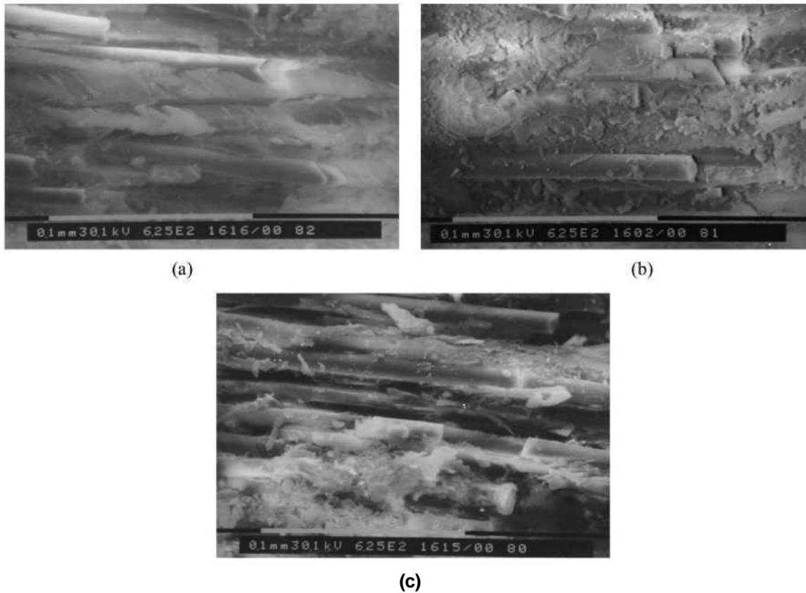
Fig. 9. SEM micrographs of GF/EP, composite eroded with steel balls of diameter = 300-500  $\mu$ m;  $v = 45 \pm 5$  m/s; exposure time = 180 s; impingement angle = 60° (a) 0° (b) 45° (c) 90° fibre orientations.
