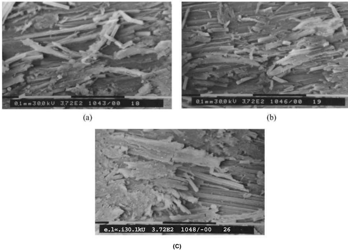
Fig. 8. SEM micrographs of CF/EP, composite eroded with steel balls of diameter = 300-500  $\mu\text{m}$ ;  $v = 45 \pm 5$  m/s; exposure time = 180 s; impingement angle = 60° (a) 0° (b) 45° (c) 90° fibre orientations.
