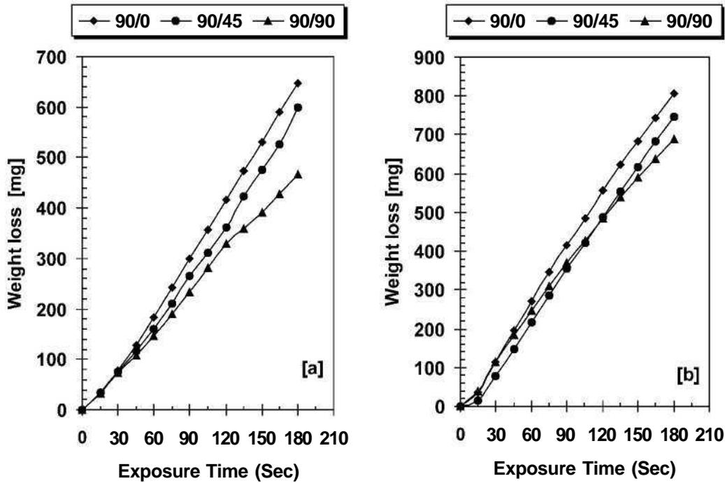
Fig. 5. Weight loss as a function of exposure time (a) CF/EP (b) GF/EP (impingement angle = 60°; v = 45 ± 5 m/s; steel balls diameter = 300-500 μm).
