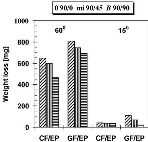
Fig. 6. Comparison of weight loss at different impingement angles for CF/EP and GF/EP (v = 45 ± 5 m/s; steel balls diameter = 300-500 μm; exposure time = 180 s).
