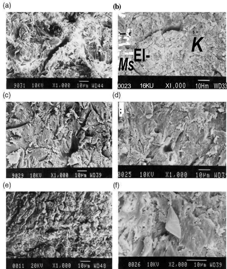
Fig. 5. SEM micrographs of eroded surfaces of aromatic PA under different condition: (a) and (b)  $a = 30^\circ$  and  $v = 140$  m/s; (c)  $a = 90^\circ$  and  $v = 140$  m/s; (d), (e) and (f)  $a = 30^\circ$  and  $v = 80$  m/s.
