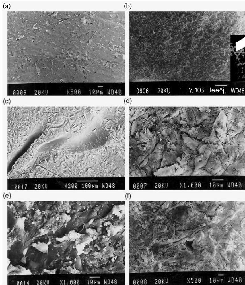
Fig. 3. SEM micrographs of eroded surfaces of PA 66/610 under different condition (a) surface farthest from the eroded zone; (b) and (c)  $a = 30^\circ$  and  $v = 140$  m/s; (d) and (e)  $a = 90^\circ$  and  $v = 140$  m/s; and (f)  $a = 90^\circ$  and  $v = 80$  m/s.
