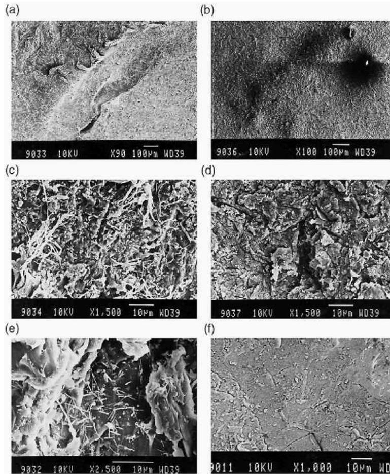
Fig. 4. SEM micrographs of eroded surfaces of PA 11 under different conditions (a), (b) and (c)  $a = 30^\circ$  and  $v = 140$  m/s; (d) and (e)  $a = 90^\circ$  and  $v = 140$  m/s; and (f)  $a = 90^\circ$  and  $v = 80$  m/s.
