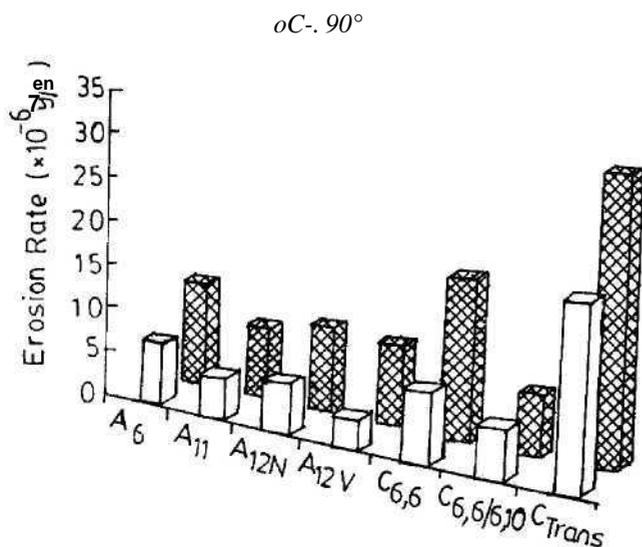
Fig. 2. Histogram showing the steady state erosive wear rates of all the materials at two impact velocities (i.e. at 80 and 140 m/s) for 90° impacts. Unfilled, lower impact velocity and filled, higher impact velocity.
