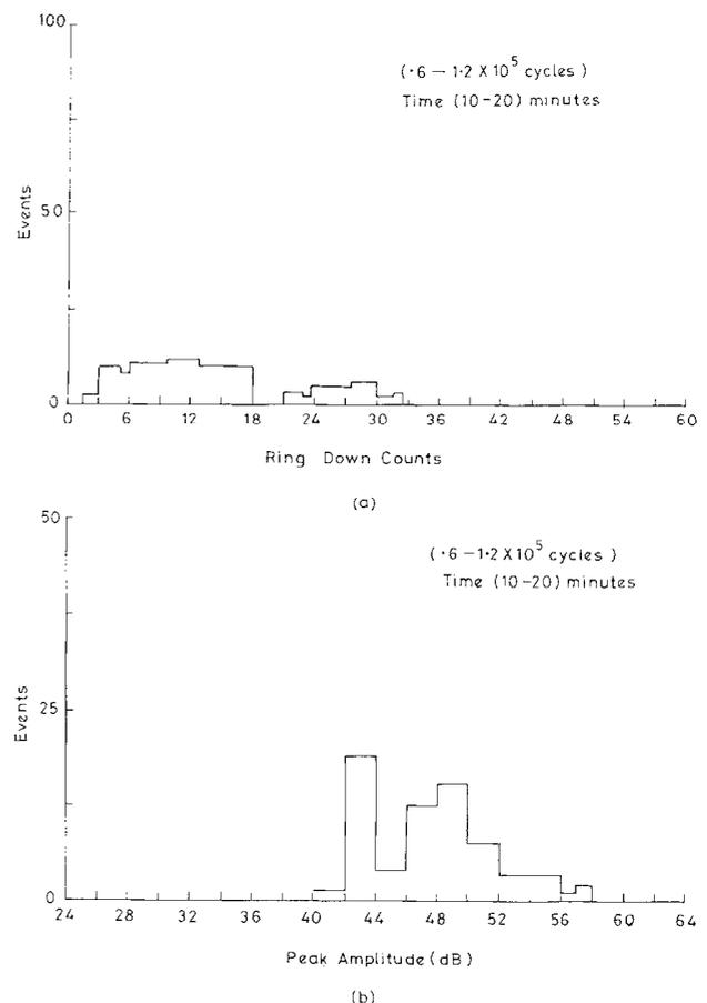
Fig 4 (a) Distribution of events by ring down counts; (b) distribution of events by peak amplitude (dB)
