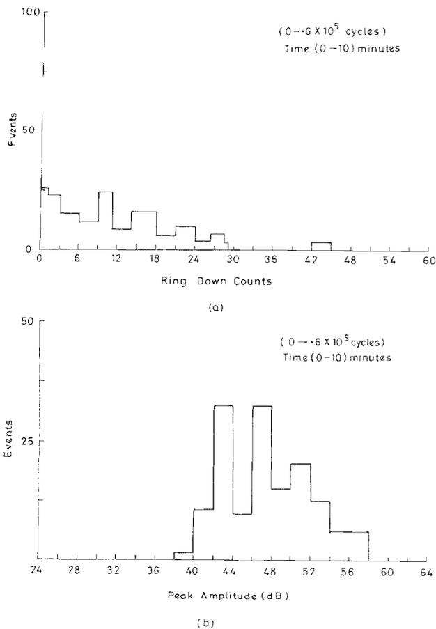
Fig 3 (a) Distribution of events by ring down counts; (b) distribution of events by peak amplitude (dB)
