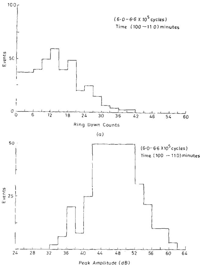
Fig 7 (a) Distribution of events by ring down counts; (b) distribution of events by peak amplitude (dB)
