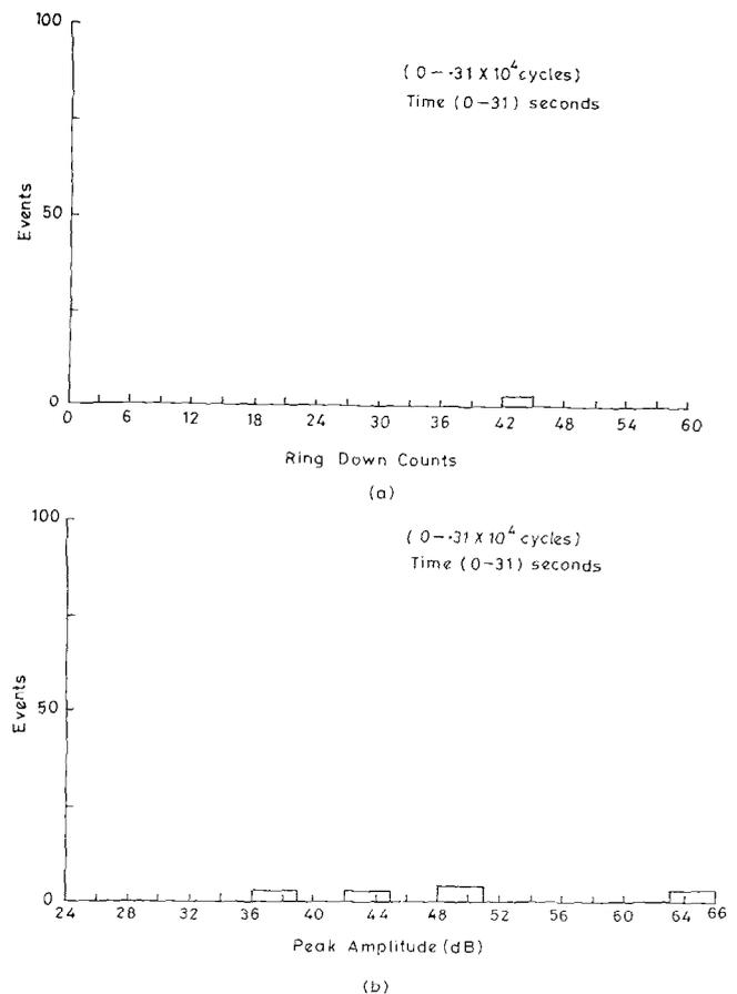
Fig 8 (a) Distribution of events by ring down counts; (b) distribution of events by peak amplitude (dB)
