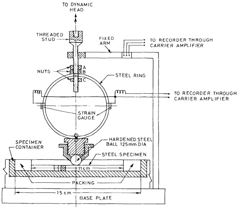
Fig 2 Set-up for cyclic loading
